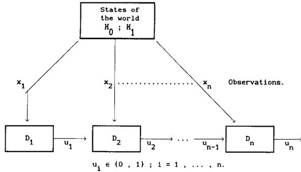
Fig. 1. Detection network in series.
